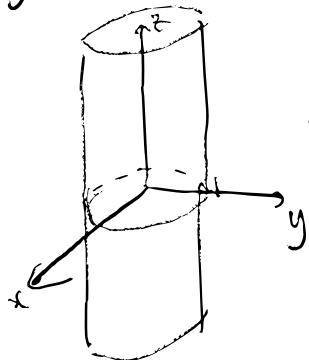
$r=1$  represents a cylinder of radius 1 that extends indefinitely along the  $z$ -axis.
