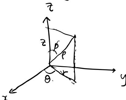
So,  $z = \rho \cos \phi$ ,  $r = \rho \sin \phi$ . Together with  $\theta = \theta$ , we get a complete set of relations between spherical and cylindrical coordinates.
