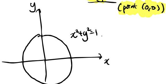
(This is because the distance between the origin and the point  $(x,y)$  is  $\sqrt{x^2+y^2}$ , by Pythagorean rule.)
